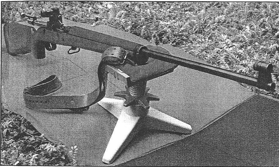
Civilian target shooting version of the Carl Gustaf M63 (M63E) imported by Parker-Hale. Better finish than the military version, but the same rifle otherwise. Still has the military Mauser trigger, but PH sights and glass-bedded.
